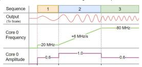
Above, the example sequence of three commands for a single core, shows a fixed 20 MHz frequency with 60% amplitude in step 1, a 10 seconds frequency ramp with 6 MHz/s slope and full 100% amplitude in step 2 and finally, in step 3, a fixed 80 MHz frequency with 50% amplitude. Each step consists of only 3 to 4 single line commands to set the mode, frequency, amplitude and timing.
