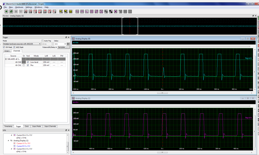
Figure 5: Another example of using the AND trigger function with an inverted logic element (low Level mode on Ch0). This triggers when a missing pulse occurs in Ch0 compared with the pulse train on Ch1.
